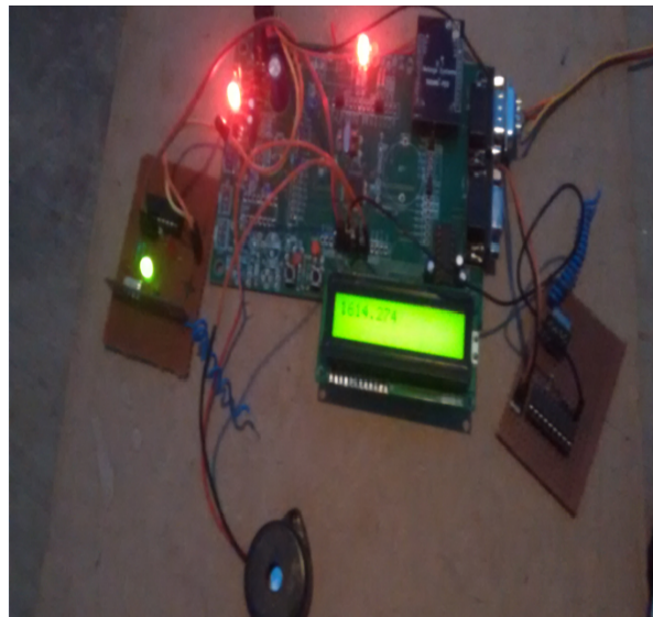
Fig. 9 Output from ZigBee modem connected to the PC in control room
