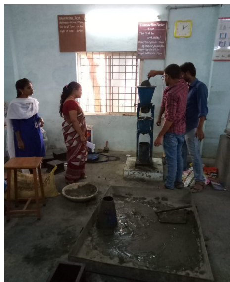
Fig 3: Conducting workability tests
