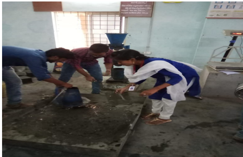
Fig 2: Conducting workability tests
