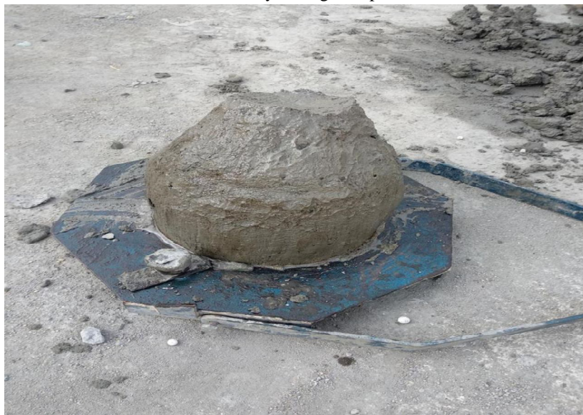
Fig. 3 slump cone result
