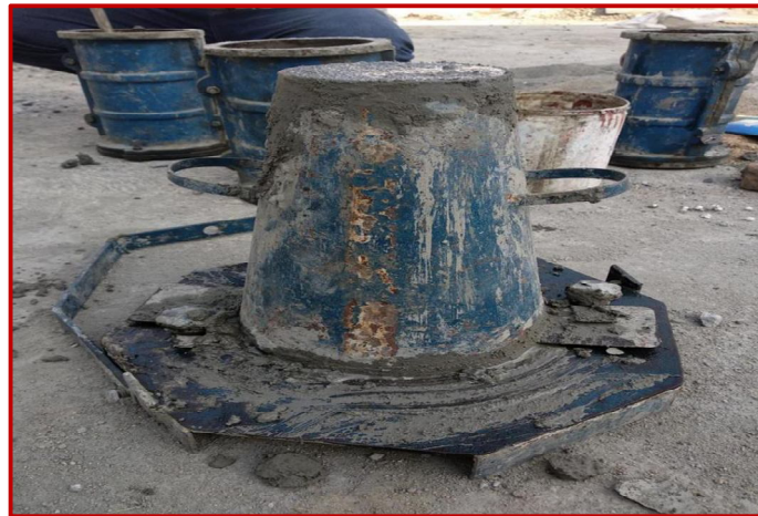
Fig.2 slump cone test
