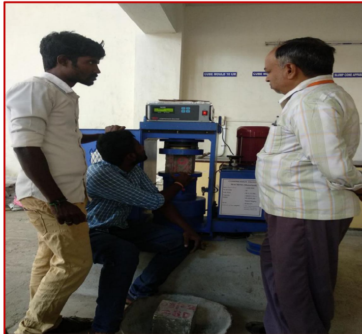
Fig. 4 compressive strength test
