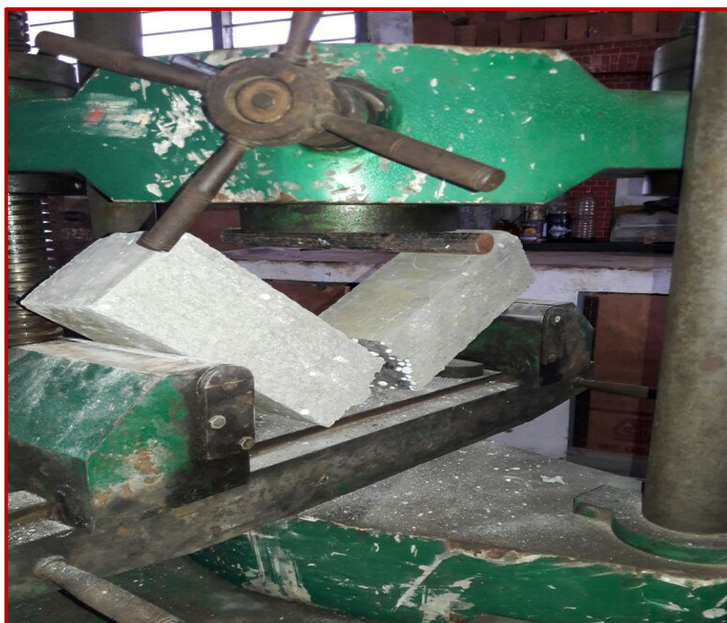
Fig.9 failure of flexural strength test
