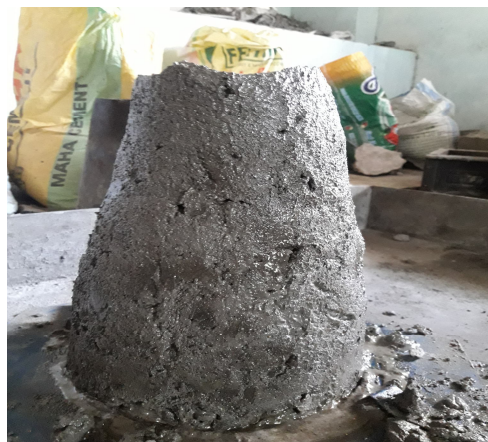
Fig 4: slump cone test
