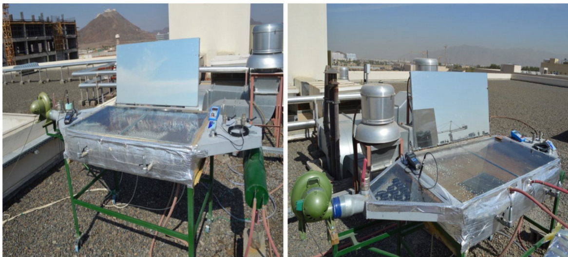
Figure 5 Experimental Test Rig (a) without solar air heater (b) with solar air heater. [5]
