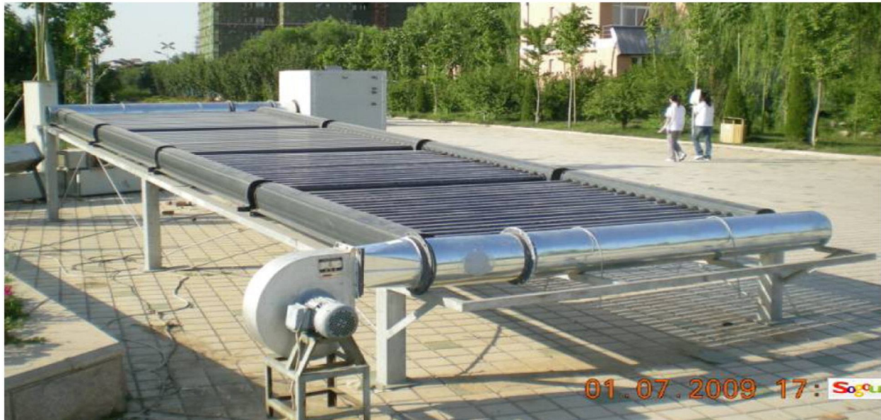
Figure 9 Photograph of solar desalination pilot plant. [9]
