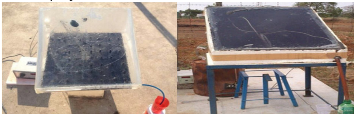
Figure 7 Experimental setup (Acrylic solar still and galvanized iron solar still) [7]
