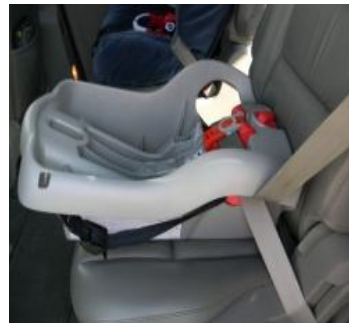
Fastening of CRS to the cars with seat belts
