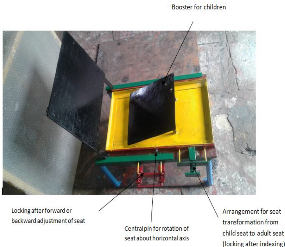
Fig. 4 Proposed rear car seat structure
