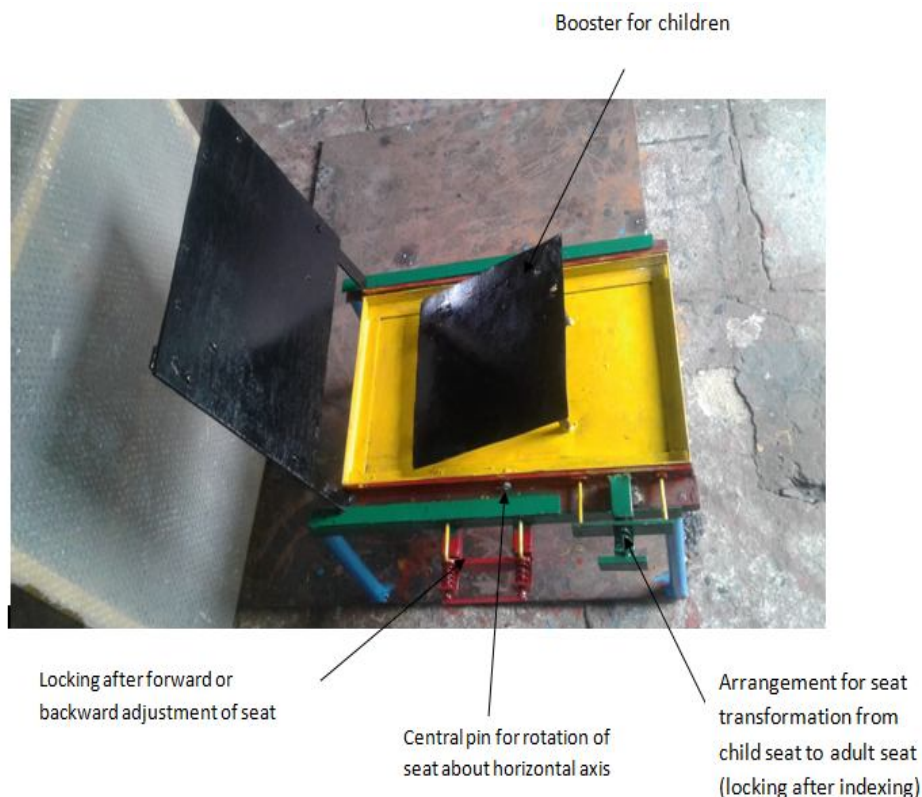
Fig. 4 Proposed rear car seat structure
