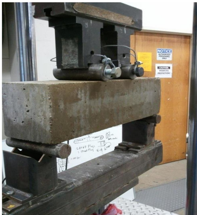
Fig. 8 Experimental setup for testing of beams
