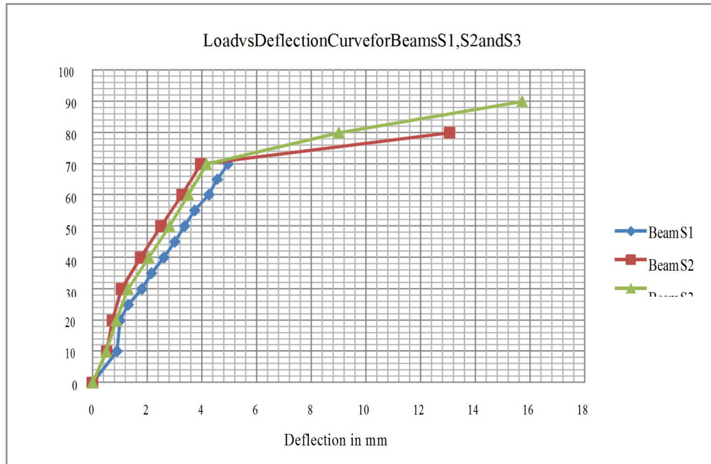
Fig. 10 Load vs Deflection Curves for Beams S1, S2 and S3.
