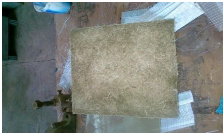
Fabricated banana fiber composite
