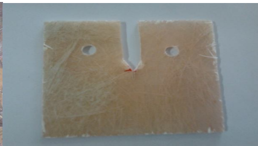
Fabricated GFRPC CT test specimen
