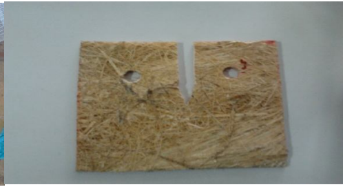
Fabricated BFRPC CT test specimen
