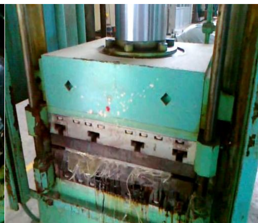
Composite fabrication in compression machine
