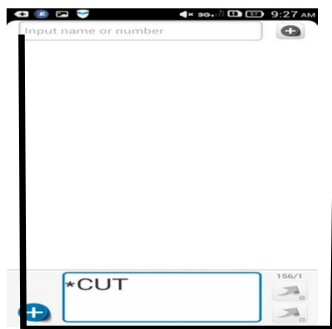
Figure 4.3: Commands to disconnect power
