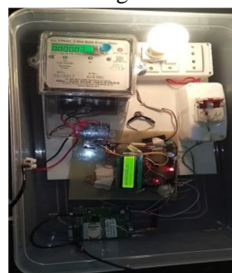
Fig5.3: set up showing the total units consumed
