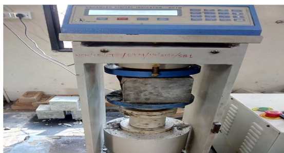
Fig no. 4.testing of cube
