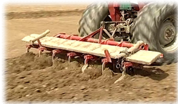
Fig: 2(c) Soil Pulverization by Cultivator Operation
