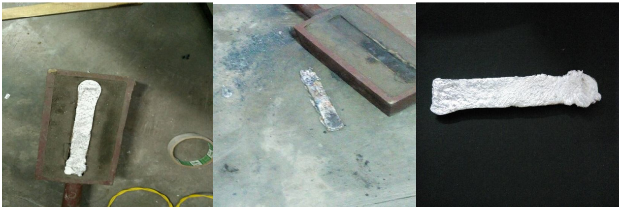
Fig. 9 Solidification of composite into the mould
