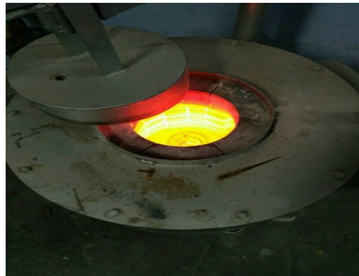
Fig. 8 Melting in Stir casting process
