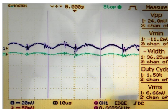
Fig 4.4 Inverter Neutral Voltage
