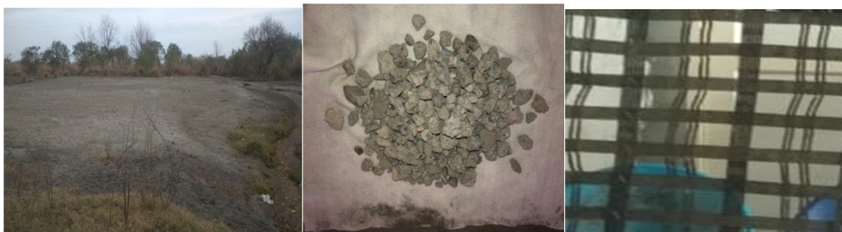
Fig. 2 Pond ash field (in thermal power plant), recycled aggregates (From Construction & Demolition waste) and Geogrid
