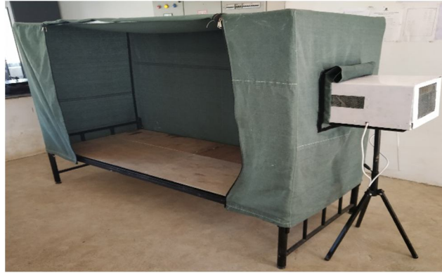
Figure 5: Cot covered with cloth and ac unit Confined area: 192×82×151 cm
