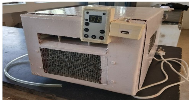
Figure 3: Air Conditioner Unit Unit dimension: 42×30×23 cm
