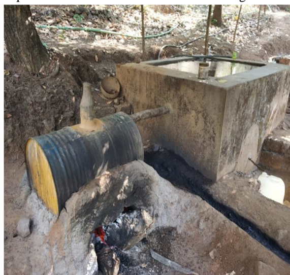
Fig-11 Distillation of ethanol collected in the tank.
