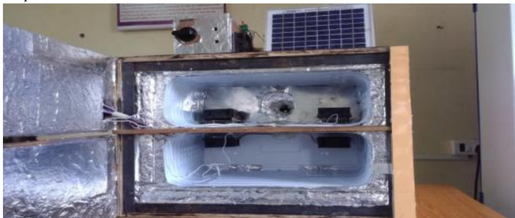
Figure 7. Designed Thermo-electric Heating & Cooling system.
