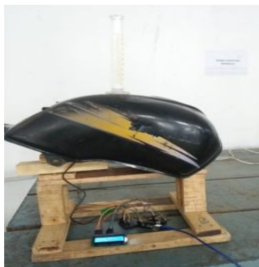
Fig.4 Mounting of measuring flask on tank
