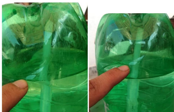
Fig 4. Before and after supply of hydrogen during downward water displacement.
