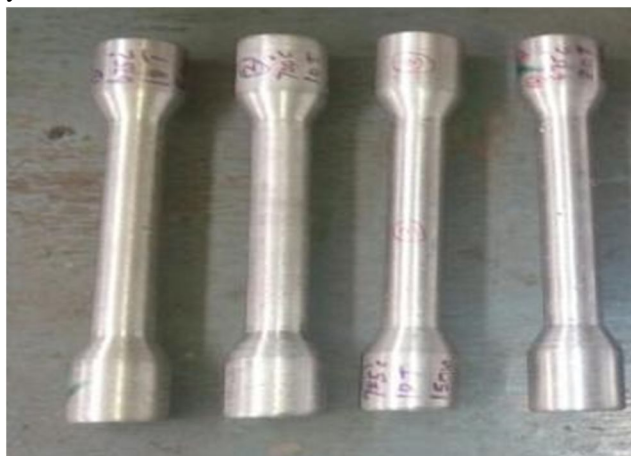
Fig. 2. Tensile Test samples
