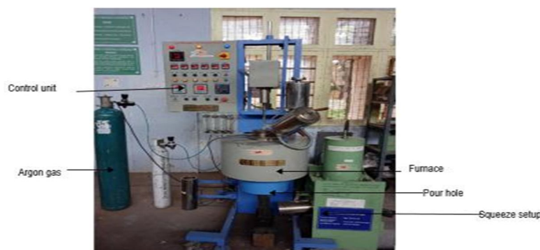
Fig. 1 Squeeze casting setup
