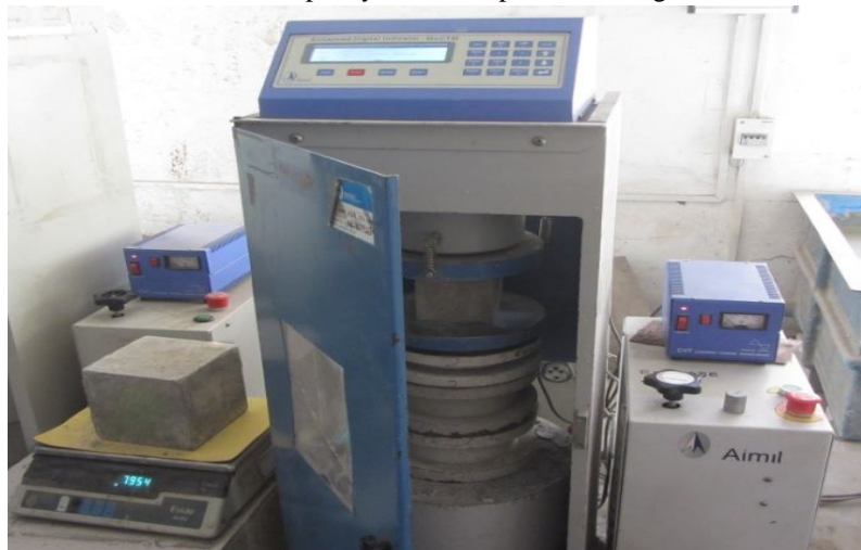
Figure 2 Compressive testing machines
