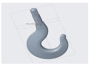
Crane Hook Geometry and model
