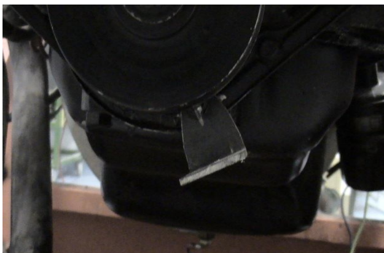
Figure 9. Setting a reference & triggering signal for cylinder #1
