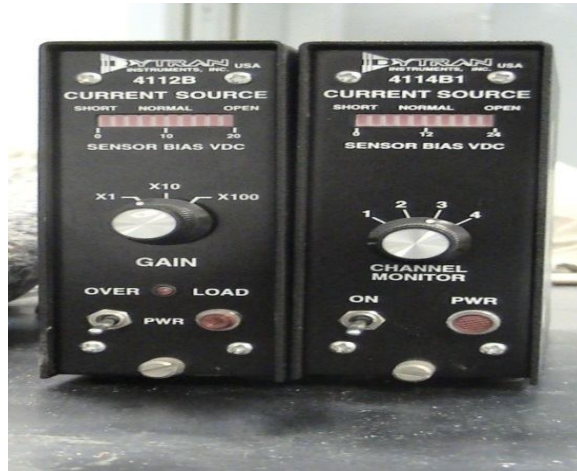
Figure 7. Charge amplifier for vibration sensor and cylinder pressure sensors
