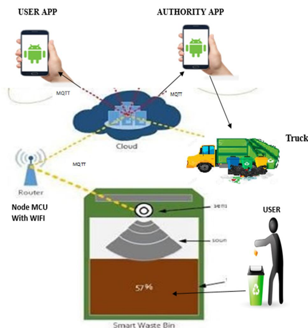
Fig 2: Smart Bin with Ultrasonic Sensor
