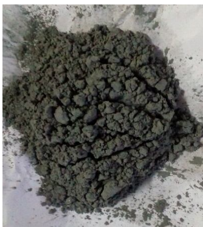
Fig: 2 Preheated cotton shell ash (CSA)
