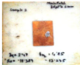
Fig3. The rectangular patch antenna without triangular section.
