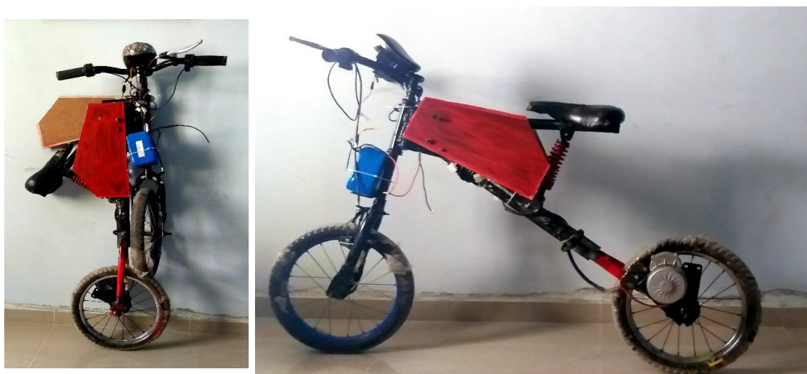
Figure 11 folded and unfolded Electric bike
