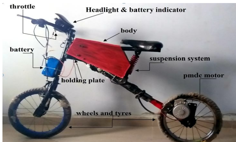
Figure1: key components of Foldable electric bike.
