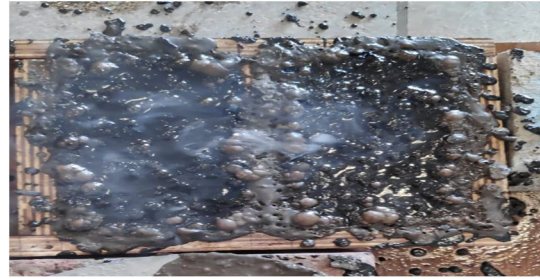
Figure 7 Hot mix poured in mould
