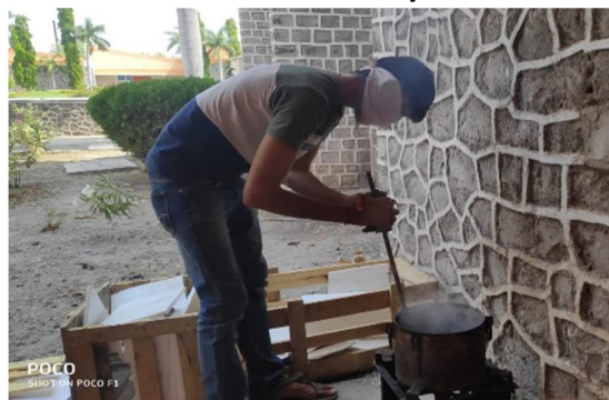
Figure 6 Melting waste plastic
