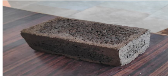
Figure 8 Paving block after removing mould
