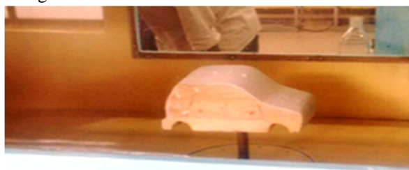
Fig. 2 Arrangement of Prototype in test section
