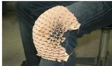
Fig. 15. Knee-cap made up of auxetic network
