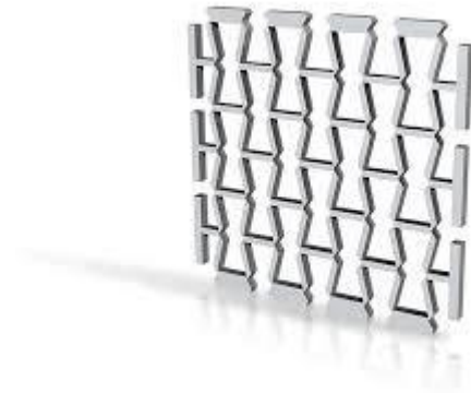
Fig. 6. Bow-tie network of auxetic materials
