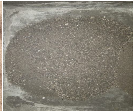
Fig. 3: Sand passing through 4.75mm sieve
