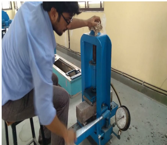
Fig.3 Flexural Strength Testing of Beam Specimen
