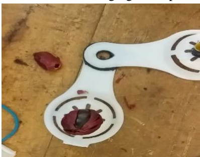
Figure 3.5: Nutmeg placing mechanism
