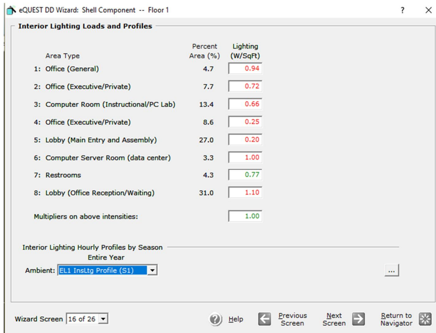
Figure 4: Screenshot of Lighting Load input screen
