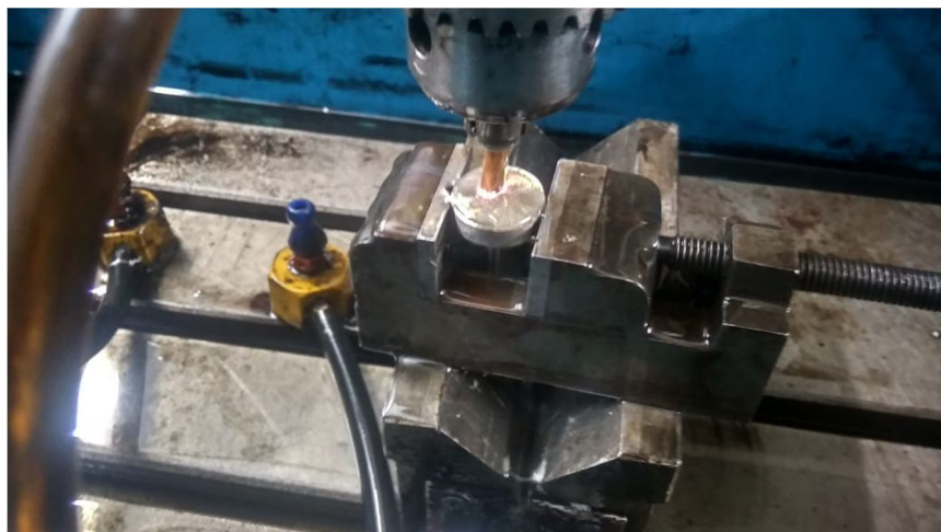
Fig. 1: Machining of EN-31 on ZNC EDM by copper tool
