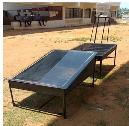
Figure 10: Solar Desalination Unit
