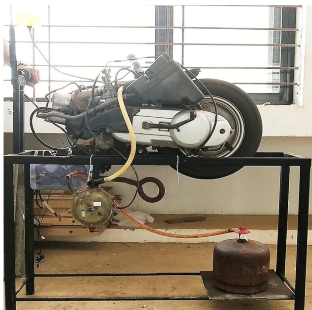
Fig.2 Single cylinder spark ignition engine connected with LPG
