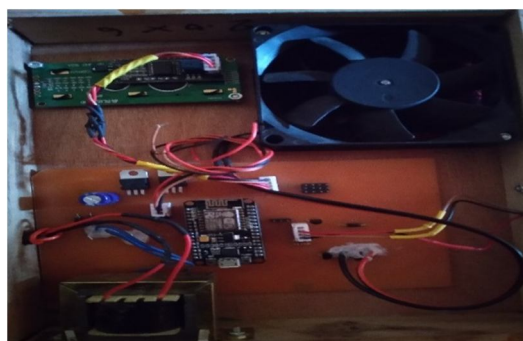
Figure 3:- Experimental setup for IOT Based Smart Air Purifier
