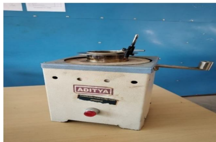
Fig 12: Claveland Flash and Fire point Apparatus
