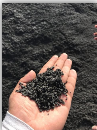
Fig. 1 Artificial Manufactured Sand
