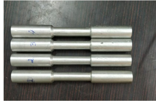
(a) Specifications of the standard tensile test sample (b) Machined Samples Figure 4. (a) Specifications of the standard tensile test sample (b) Machined Samples
