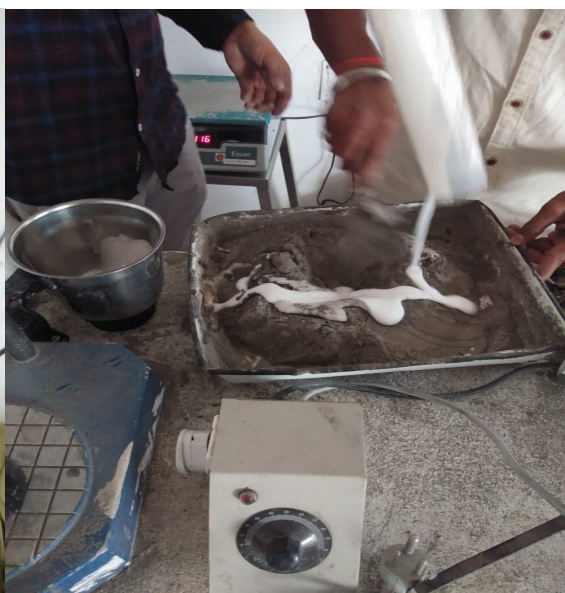
fig4: mixture of fly ash and cement with foaming agent
