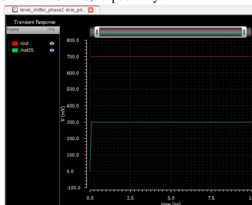
Figure 1.15 Transient response of conventional dual current mirror based level shifter
