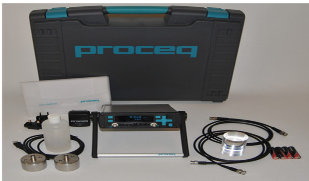
Fig.6 Ultrasonic Pulse Velocity Testing Instrument
