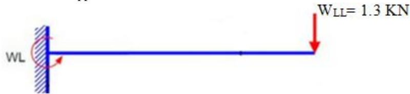
Fig. 3.6: Live load distribution on cantilever steps.
