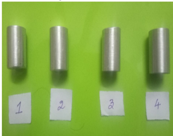
Fig 8 Corrosion tested samples
