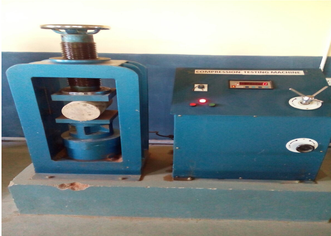
Figure 5.2 Split tensile strength of cylinder setup
