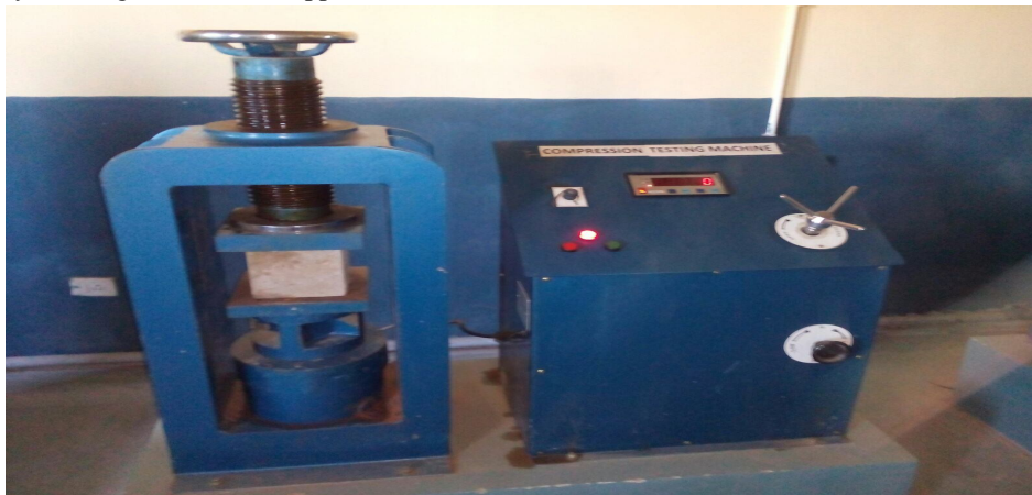
Fig. 5.1 Compressive strength of concrete cube setup
