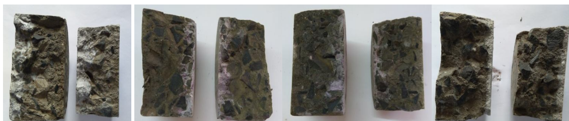
Figure-10: Silver Nitrate test for Chloride permeability in concrete for all four types of cement mix S1 to S4 (left to Right).
