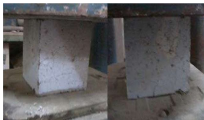
Fig. 4.1: Concrete specimens subjected to 300°C and 600°C
